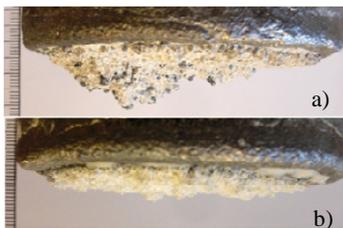
Figure 4. 'Unsuccessful' gravity experiments with 150 mm of head showing metal frozen over the filter with: (a)  $\sim 18$  mm of metal penetration, using a 50 PPI CFF and (b) less than 7 mm of metal penetration, using a 80 PPI CFF.
