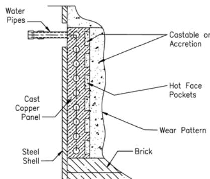
Figure 2. Water cooled slag furnace copper cooler with a hot face pattern [3].
