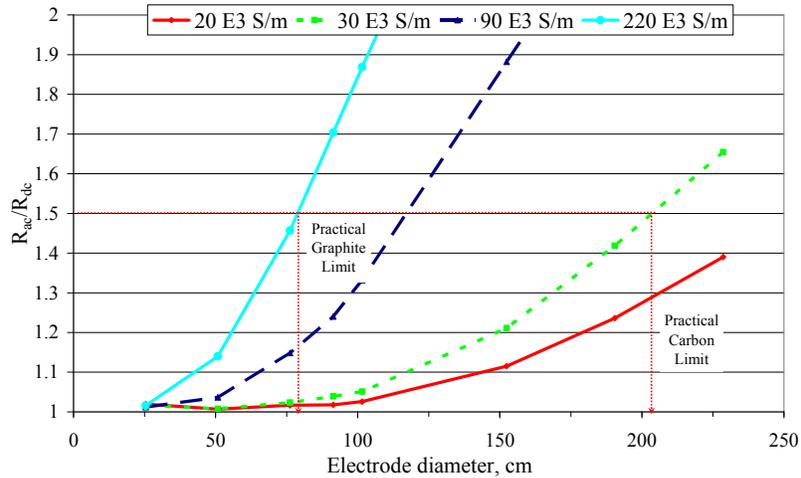
Figure 4. Ratio of  $R_{ac}/R_{dc}$  for electrodes at 50 Hz.
