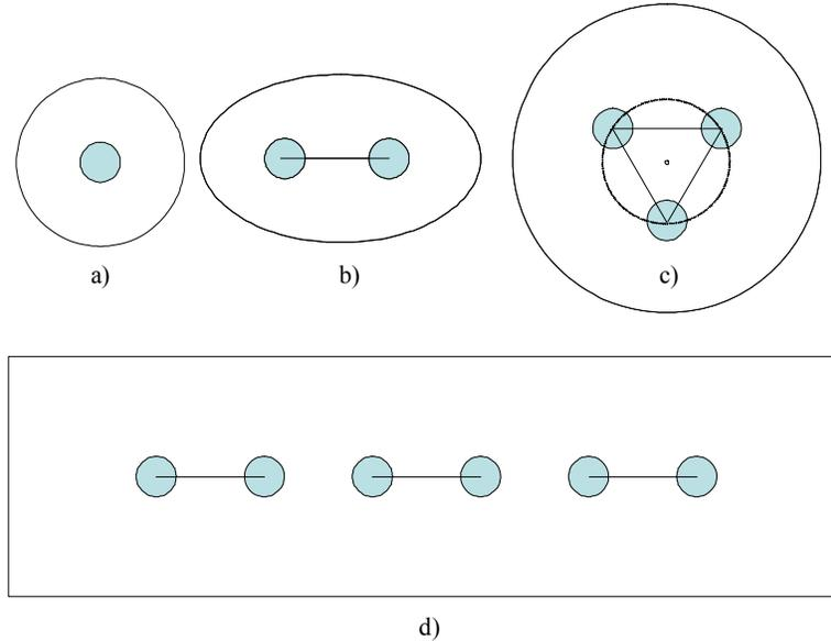
Figure 3. Typical electric furnace electrode and furnace body arrangements: a) single top entering electrode (1-phase), b) two electrodes (1-phase), c) three electrodes (3-phase) and d) six-in-line electrodes (3-single phase).
