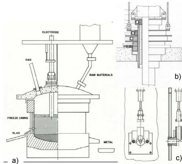
Figure 1. Overview of some furnace details. a) Elkem Multi-Purpose Furnace<sup>®</sup>, b) electrode seal, and c) slag flow controller [2].
