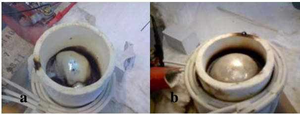
Figure 6. The multi-layer coil (Coil 2) with a magnetic flux density of a) \sim 0.20 T, and b) \sim 0.12 T.
