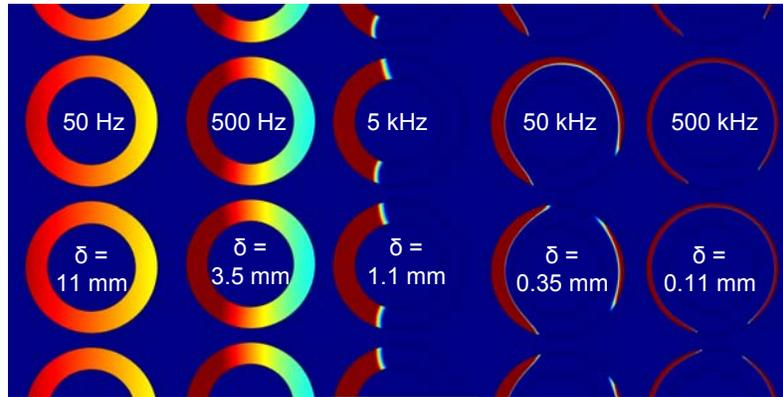
**Figure 3.** COMSOL<sup>®</sup> Results Showing Relative Current Distribution for Frequencies Ranging from 50 Hz to 500 kHz, (The Coil Centre Line is on the Left Side of the Conductors).
